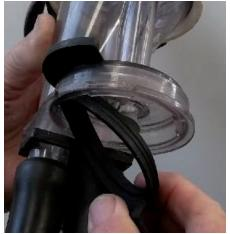
**Step 3.** Remove the flask seals from the meters, wash and leave in the bucket provided.
